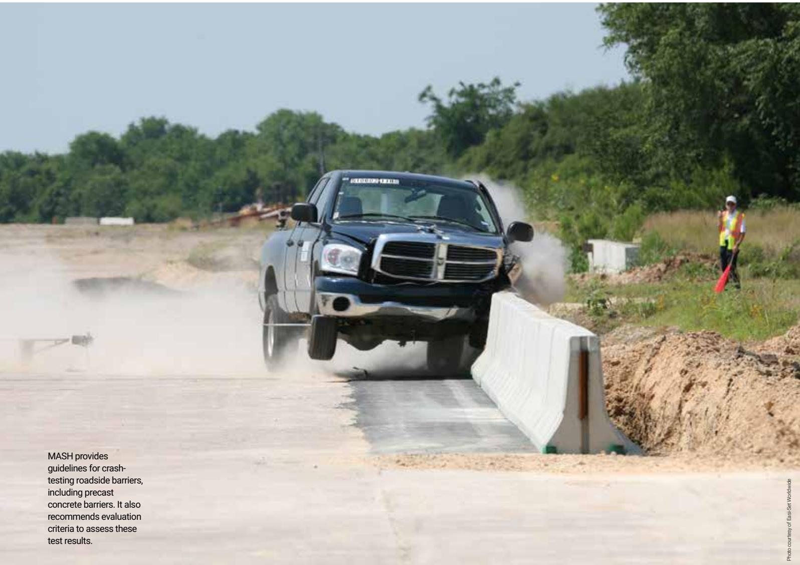
MASH provides guidelines for crash-testing roadside barriers, including precast concrete barriers. It also recommends evaluation criteria to assess these test results.
